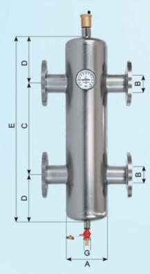
The **SRG Multifunctional Hydraulic Separator** is a device designed for heating and cooling systems. It serves to separate the primary and secondary circuits connected to it, ensuring their independence and compensating for flow rate differences between the circuits.
