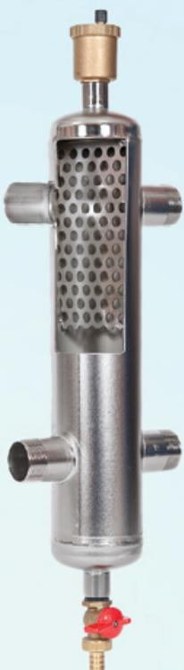
A further function of the hydraulic separator is performed by the sludge separator inside the device. It allows the separation and collection of impurities in the system, which are removed by means of the drain valve in the lower part (which can be opened when the system is running).
